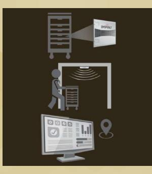
Attach Impinj-powered RAIN RFID tags to supplies and medications.
